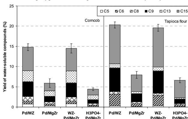
**Figure 2.** Yield of water-soluble C<sub>5</sub>-C<sub>15</sub> organic compounds from the integrative hydrolysis/dehydration/aldol-condensation/hydrogenation of corn cob and tapioca flour in the presence of various catalyst systems [2].
