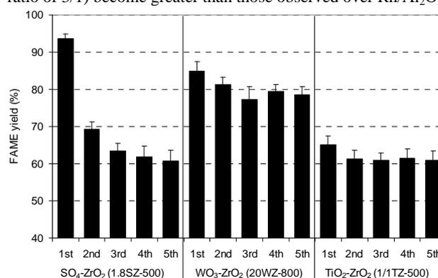
**Figure 3.** Reusability testing (in 5 reaction cycles) of 1.8SZ-500 (1 wt%), 20WZ-800 (0.5 wt%) and 1/1TZ-500 (1 wt%) toward the esterification of PFAD at 80°C with the reaction time of 120 min and methanol to PFAD molar ratios of 6:1 [3].
